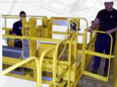
ACCESS GATES w/ SAFETY INTERLOCKS
