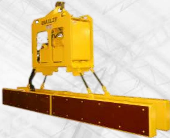
HYDRAULIC FLUE WALL STRAIGHTENER (THREE INDEPENDENTLY DRIVEN CYLINDERS TO RE-ALIGN REFRACTORY WALL BRICKS)
