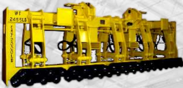
PNEUMATIC FLUE WALL CLEANER (WIRE BRUSHES TO REMOVE COKE BUILD-UP ON FLUE WALL SURFACES)
