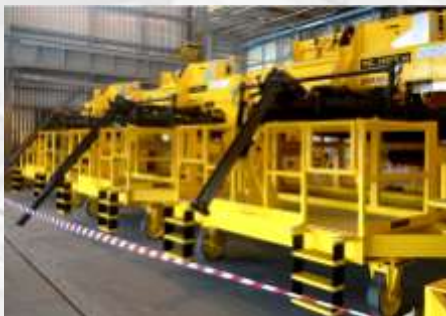
CRUCIBLE LIFTERS ON TRAILERS W/ LIDS & SIPHONS
