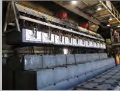
TONG TO HANDLE 12 LARGE ANODES IN STORAGE AREA
