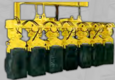
SHUFFLER GRAB TO ROTATE ANODES 90°
